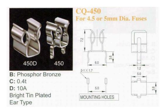
P.C. Board Mount Fuse Clips For 4.5 or 5mm Dia. Fuses
