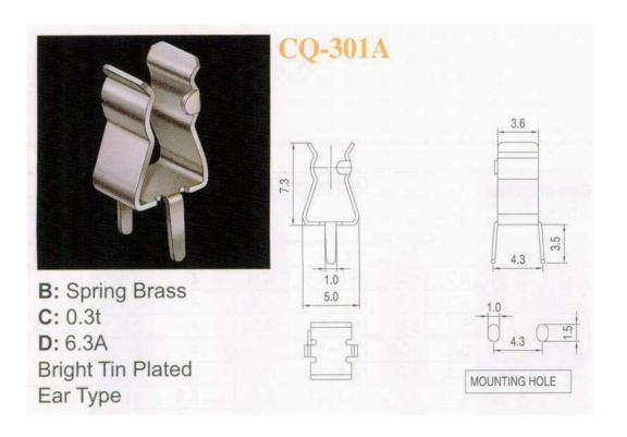
P.C. Board Mount Fuse Clips For 3.6mm Dia. Fuses
