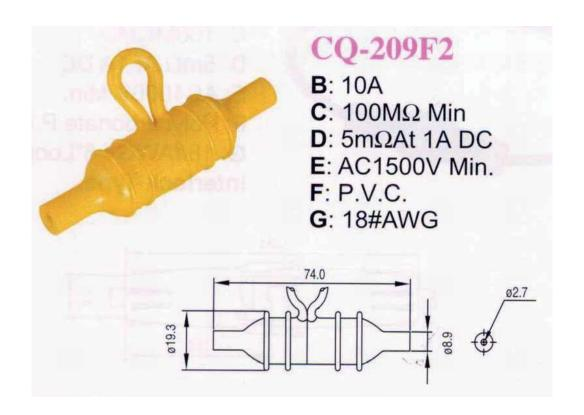
In-Line Fuse Holder For 1/4"x1-1/4 (6.3x32mm or 6.3x30mm) Fuses
