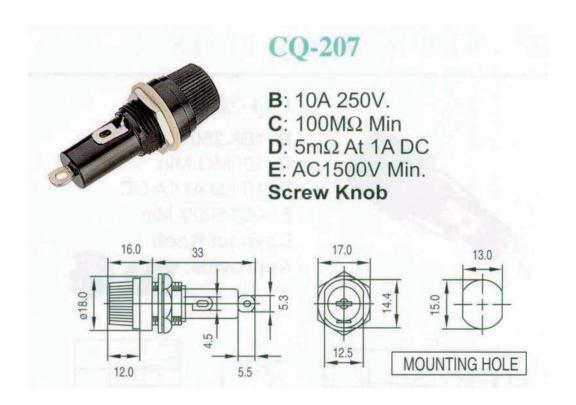
Panel Mount Fuse Holder For 1/4"x1-1/4(6.2x32mm) Fuses
