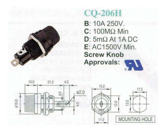
Panel Mount fuse Holder For 5x20mm Fuses \*Rated Current : 10A/250V\*Insulation Resistance At 500VDC :  $100M\Omega$ Min \*Contact Resistance :  $5m\Omega$  At 1ADC\*Dielectric Strength For 60 Sec : AC1500V Min. \*Approvals : RU Screw Knob
