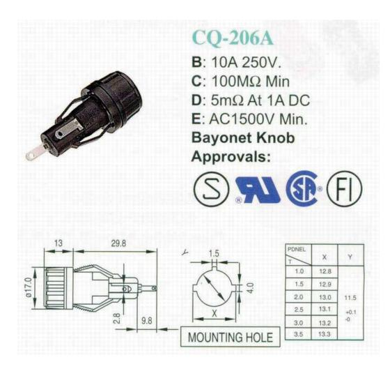
Panel Mount fuse Holder For 5x20mm Fuses \*Rated Current : 10A/250V\*Insulation Resistance At 500VDC :  $100M\Omega$ Min \*Contact Resistance :  $10m\Omega$  At 1ADC\*Dielectric Strength For 60 Sec : AC1500V Min. \*Approvals : RU,CSA
