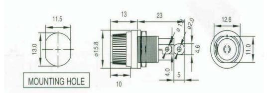
Panel Mount fuse Holder For 5x20mm Fuses \*Rated Current : 10A/250V\*Insulation Resistance At 500VDC :  $100M\Omega$ Min \*Contact Resistance :  $5m\Omega$  At 1ADC\*Dielectric Strength For 60 Sec : AC1500V Min. Screw Knob
