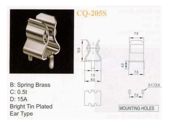
P.C. Board Mount Fuse Clips For 1/4" (6.3mm) Diameter Fuses \*Metal Material : Spring Brass \*Material Thickness : 0.5t \*Suitable Rated Current : 15A Bright Tin Plated Ear Type
