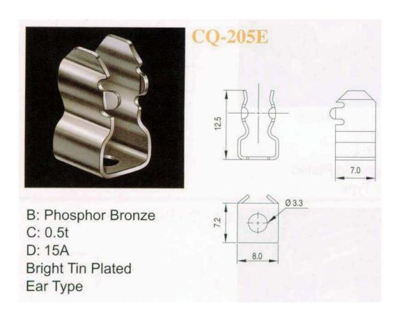
P.C. Board Mount Fuse Clips For 1/4" (6.3mm) Diameter Fuses
