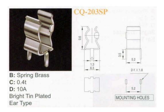
P.C. Board Mount Fuse Clips For 5mm Diameter Fuses \*Metal Material : Spring Brass \*Material Thickness : 0.4t \*Suitable Rated Current : 10A Bright Tin Plated Ear Type
