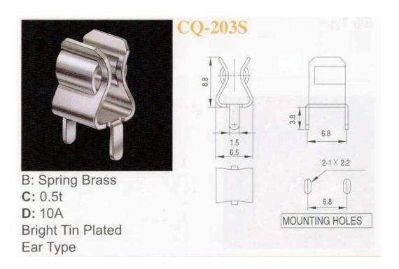
P.C. Board Mount Fuse Clips For 5mm Diameter Fuses \*Metal Material : Spring Brass \*Material Thickness : 0.5t \*Suitable Rated Current : 15A Bright Tin Plated Ear Type
