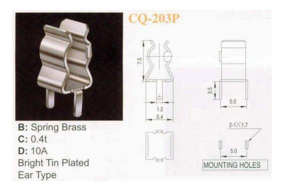
P.C. Board Mount Fuse Clips For 5mm Diameter Fuses
