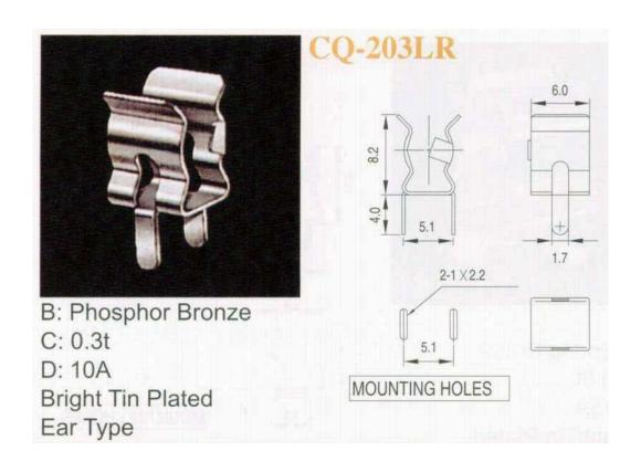
P.C. Board Mount Fuse Clips For 5mm Diameter Fuses
