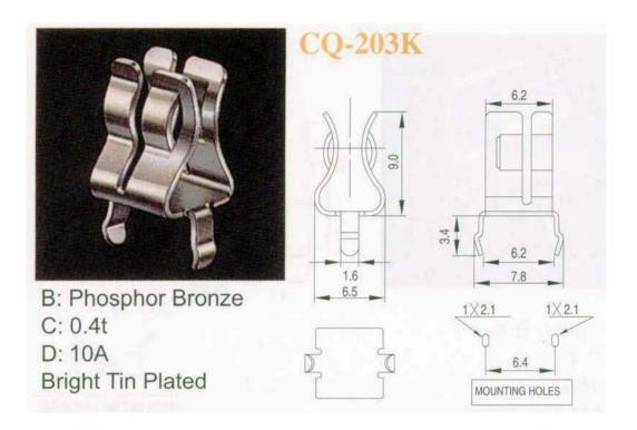
P.C. Board Mount Fuse Clips For 5mm Diameter Fuses \*Metal Material : Spring Brass \*Material Thickness : 0.4t \*Suitable Rated Current : 10A Bright Tin Plated
