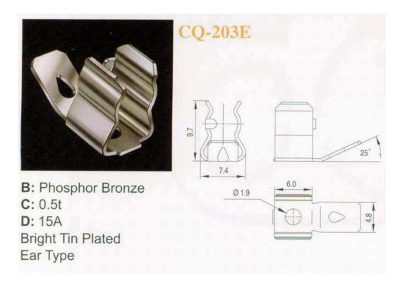
P.C. Board Mount Fuse Clips For 5mm Diameter Fuses
