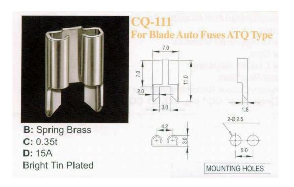
P.C. Board Mount Fuse Clips For Blade Auto Fuses ATQ Type
