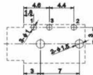
P.C.B Layout(copper-sided view)
