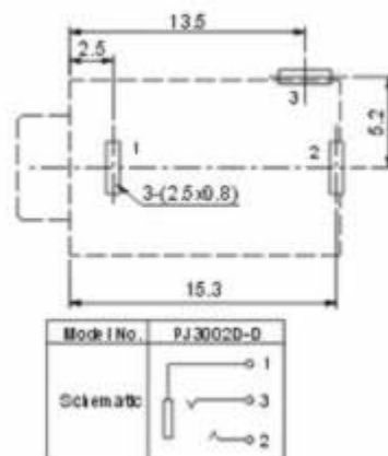
P.C.B Layout(copper-sided view)
